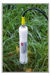
The Profile Probe measures the soil moisture profile when inserted into an access tube that has been installed in the soil
