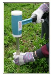
If you are inserting access tubes level with the soil surface, continue hammering until the top of the tube is just level with the soil surface.
